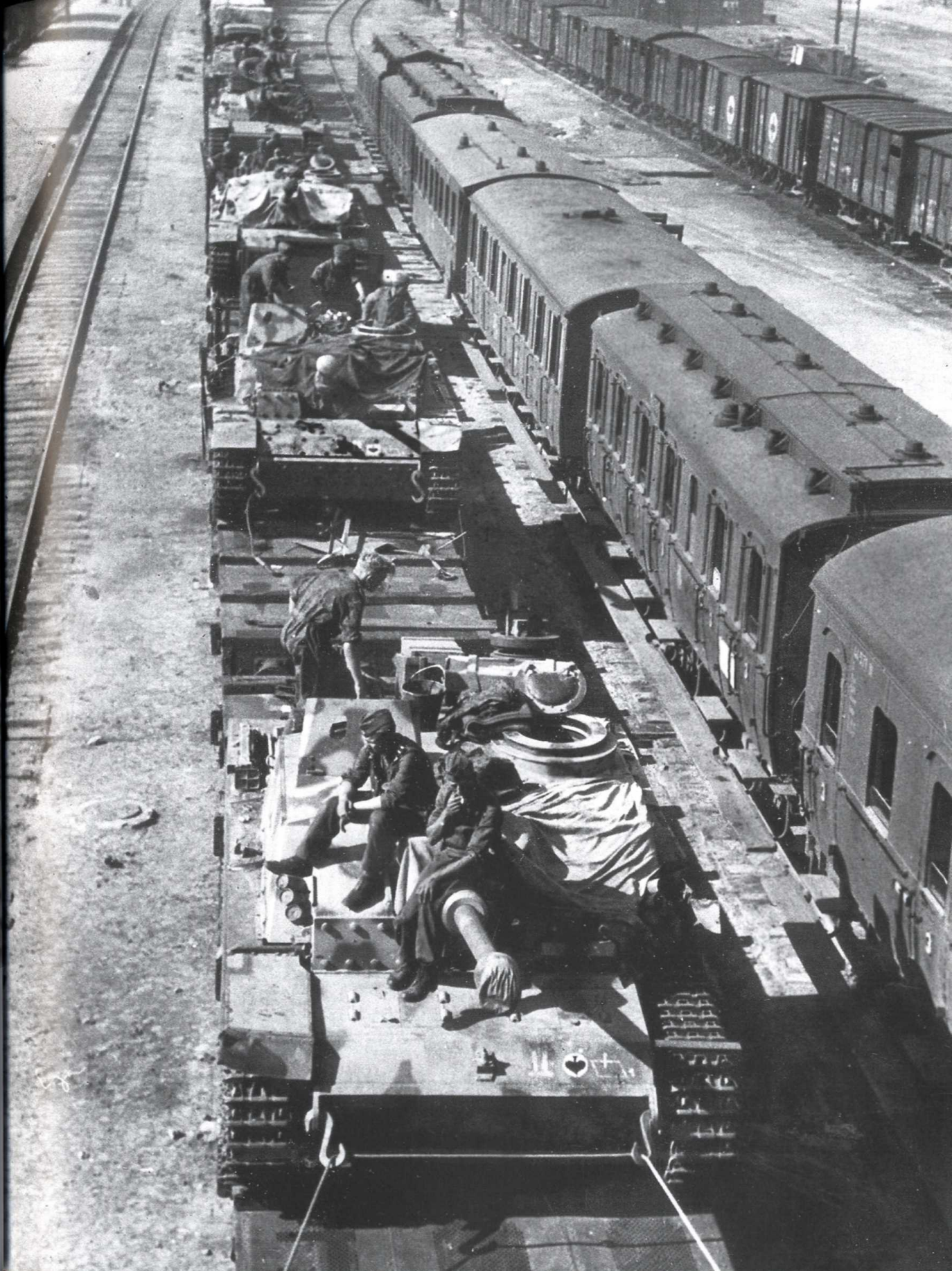
Opposite: One of the most common and practical methods of transporting armour was by rail. Here a Sturmgeschütz unit is being readied for transportation most probably to the Eastern Front. Note the smoke candle dischargers attached to the side of the vehicles superstructure.
