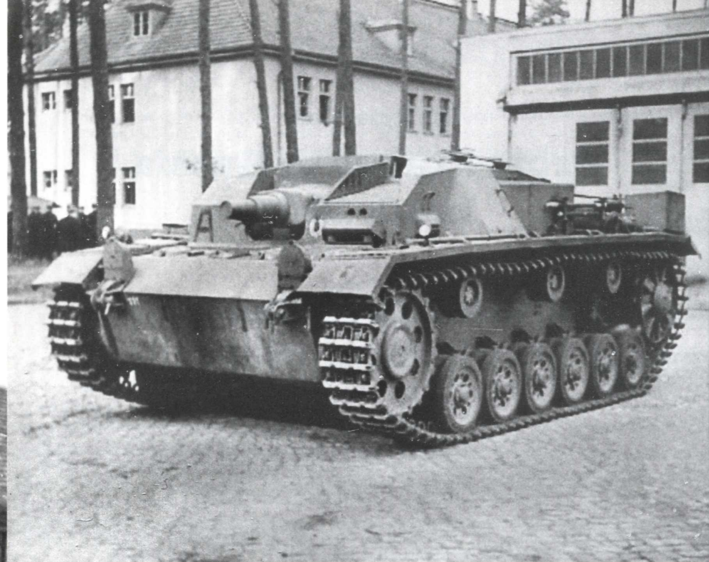
At a training ground an early StuG.III can be seen. In 1939 this vehicle rolled off the production line. It was armed with a 7.5cm KwK L/24 gun and was installed in a fixed superstructure on the chassis of a Pz.Kpfw.III tank.
