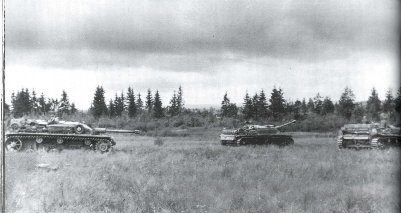
Three StuGs can be seen operating in an open field during the early summer of 1943. The assault gun in the middle is an Ausf.F/8 variant, whilst the other two are standard Ausf.F models. The Ausf.F series was the first StuG to be introduced with the longer L/43 calibre StuK40, and then the L/48 calibre weapon.
