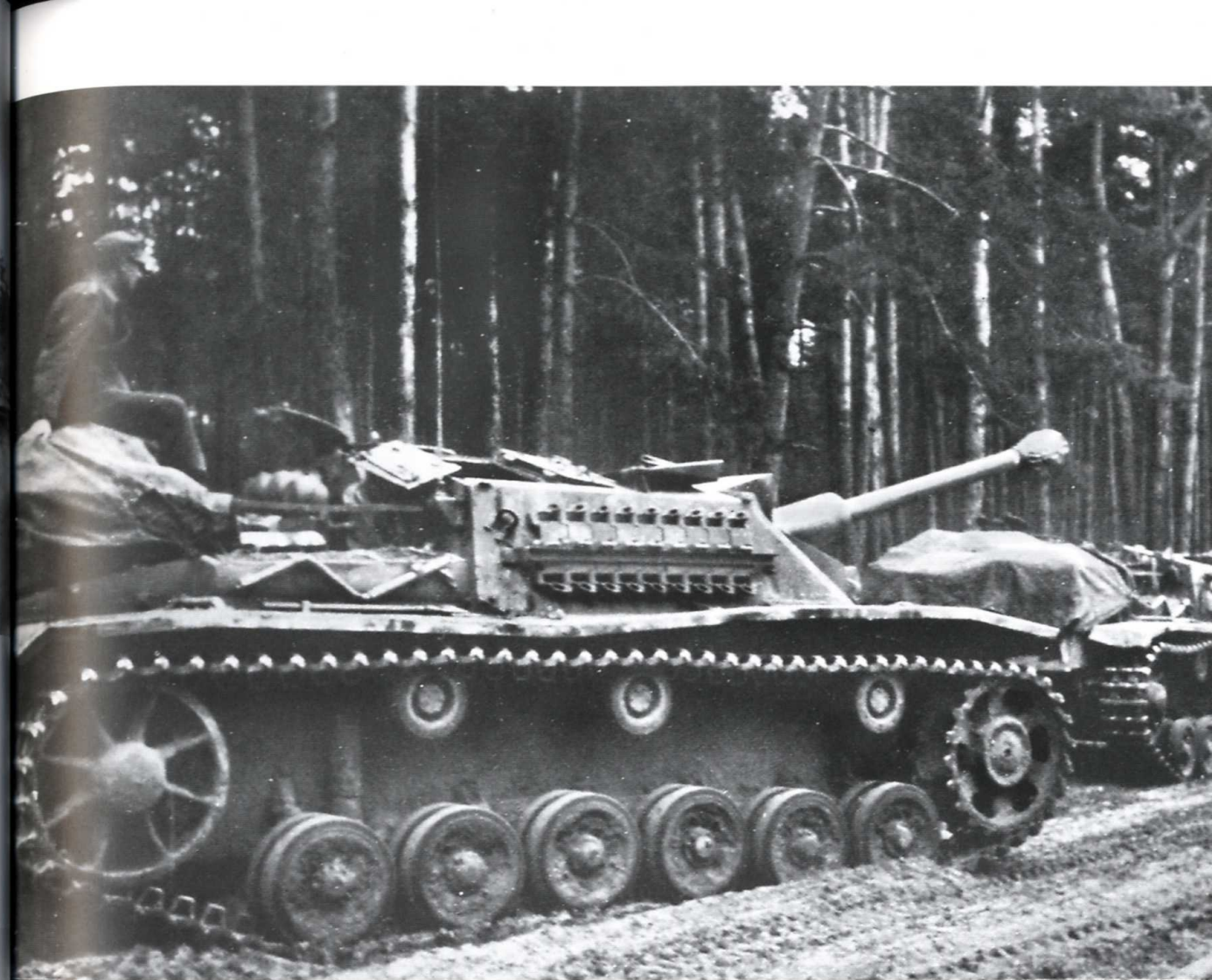
Two Ausf.G's halted on a muddy road. The StuG crews are using the forest as concealment against both aerial and ground observation. The longer barreled cannon and the modification of the frontal superstructure increased the overall weight of the vehicle to 21.3-tons.
