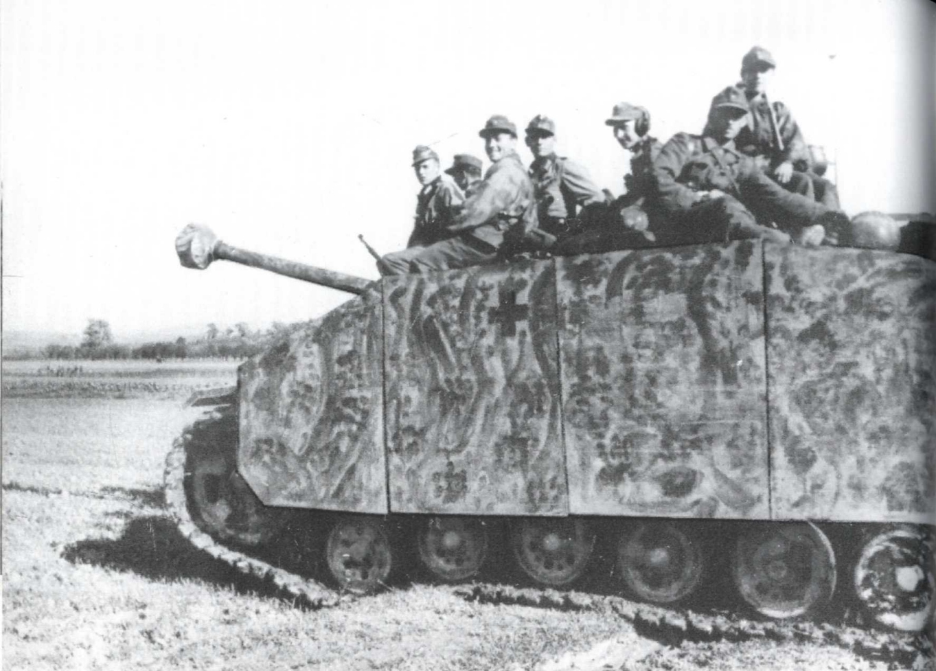
Two photographs showing a StuG.III.Ausf.G with very interesting camouflage paint. The armoured side skirt plates have been painted in a pattern of green and brown over the dark yellow sand base. Dense groups of small dots and curving streaks have also been applied. Note the factory built stowage bin attached on the rear of the engine deck.
