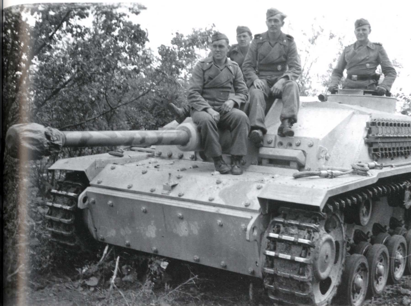
The crew pose for the camera on their early production StuG.III.Ausf.G. Note how the crew have fitted the a rack of spare tracks on the vehicles casemate side wall.
