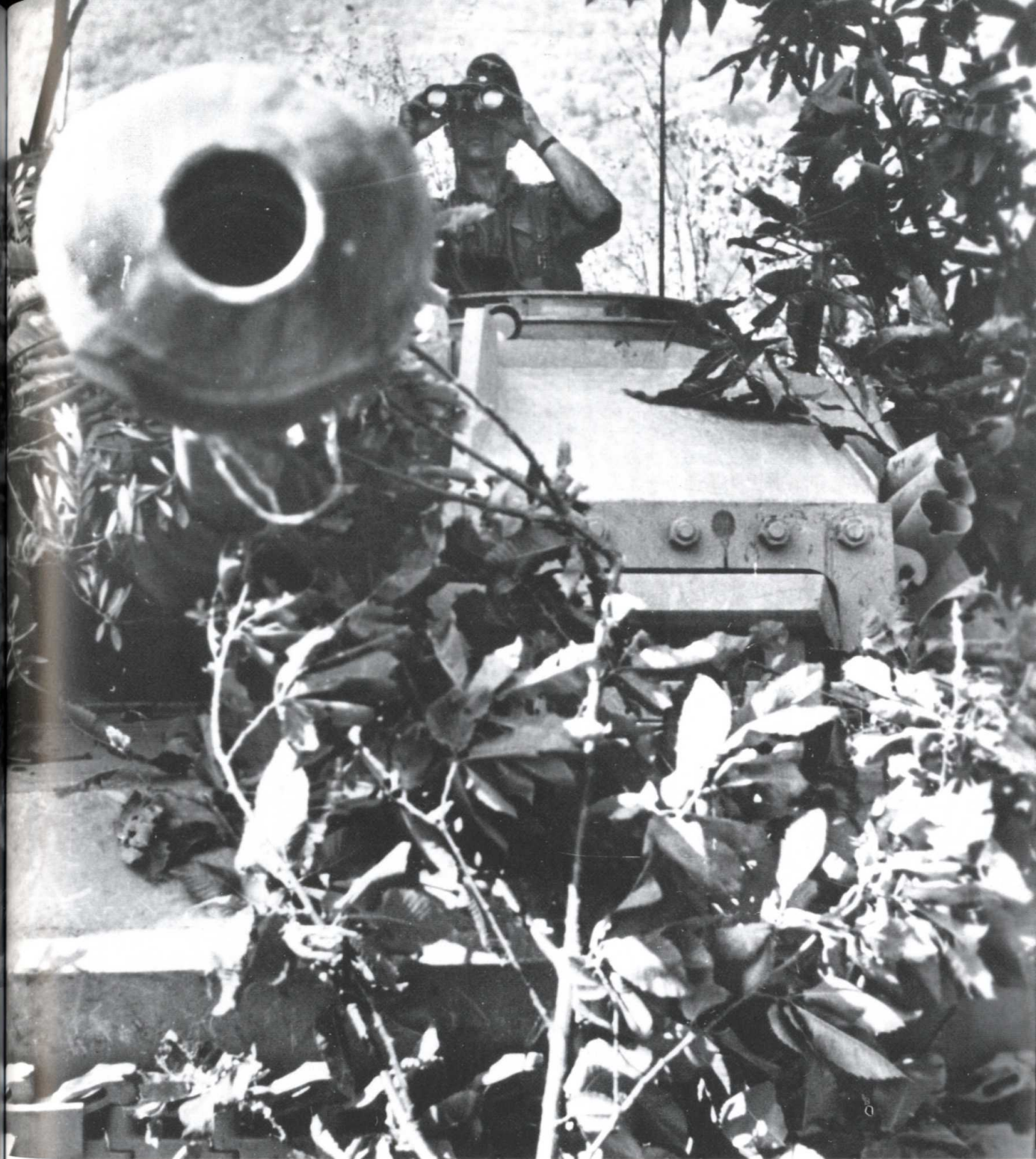
A well camouflaged StuG.III more than likely operating in Italy. Note the smoke candle dischargers attached to the side of the vehicles superstructure.
