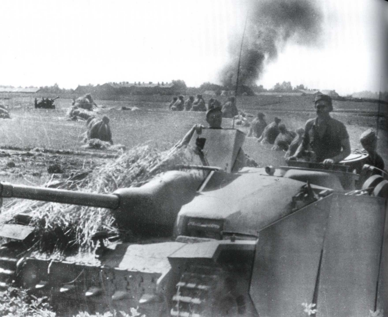
A late variant StuG.III.Ausf.G during operations in Army Group Centre in the summer of 1944, possibly during 'Operation Bagration'. Of interest is the layer of concrete on the front of the casemate in order to give the vehicle additional armoured protection.
