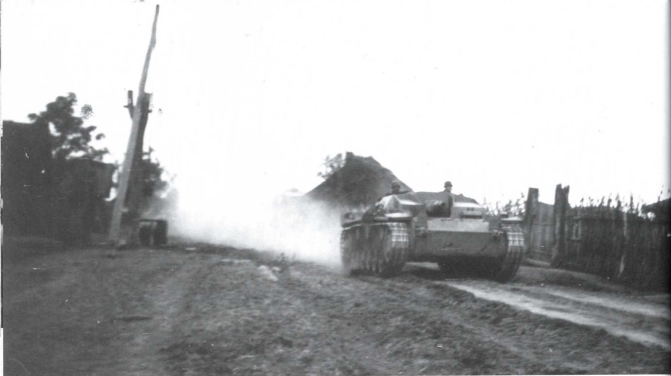
An StuG.III. Ausf.B hurtles along a dusty road during the summer of 1941 on the Eastern Front. For the invasion of Russia German factories were able to complete 548 StuG.III vehicles. The StuG had a crew of four and came equipped with a 7.5cm StuK 37 L/24 gun capable of traversing from 12.5 degrees left to 12.5 degrees right.
