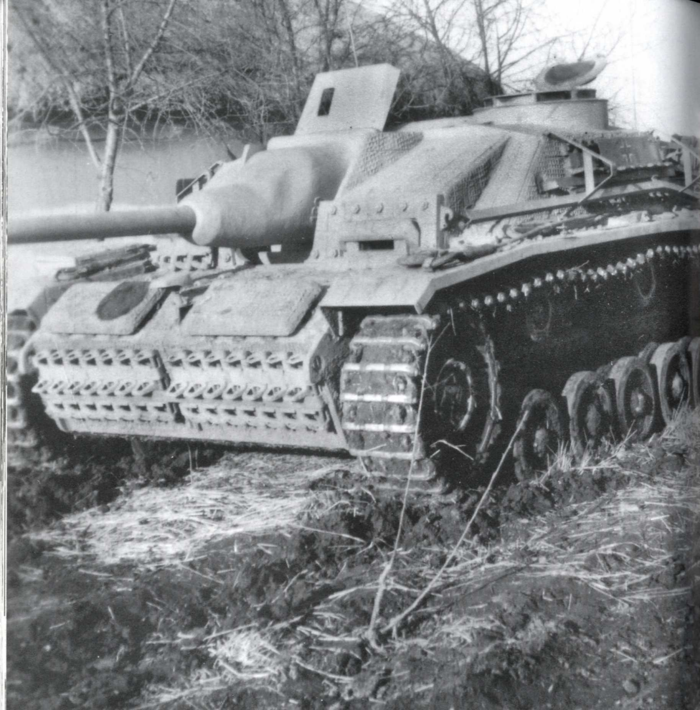
A stationary white-washed StuG.III.Ausf.G with missing side skirts can be seen in a muddy field. The vehicle has an application of Zimmerit anti-magnetic mine-paste. In September 1944 Zimmerit was discontinued as there were concerns that it was inflammable under the impact of projectiles.
