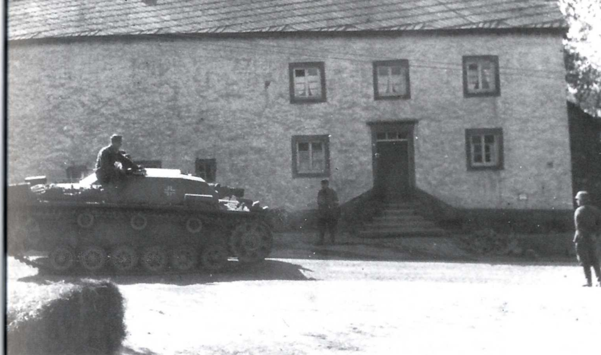
A StuG.III Ausf.A advances along a road through France destined for the front lines. This assault gun is identified as an Ausf.A because it mounts the early idler wheel and the original position of the forward return roller.
