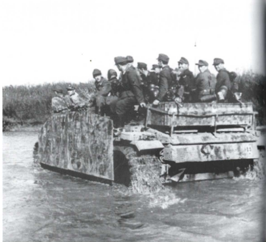
Two photographs showing a StuG.III.Ausf.G with very interesting camouflage paint. The armoured side skirt plates have been painted in a pattern of green and brown over the dark yellow sand base. Dense groups of small dots and curving streaks have also been applied. Note the factory built stowage bin attached on the rear of the engine deck.
