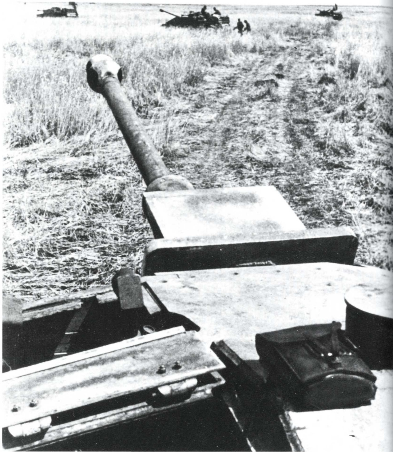
An excellent photo of a 7.5cm gun barrel of an unidentified StuG.III out on the Russian steep. Despite the longer 7.5cm barrel this assault gun was continually hard pressed on the battlefield and constantly called upon for offensive and defensive fire support, where it was gradually compelled to operate increasingly in an anti-tank roll.
