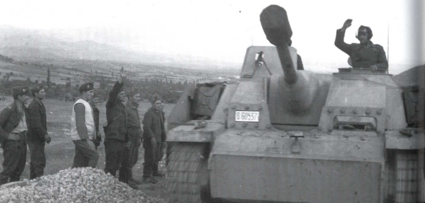
This page and opposite: Four photographs apparently showing the same Bulgarian Maybach T-III (StuG.III.Ausf.G). The vehicle registration number 'B60537' can quite clearly be indentified on both the rear and front plates of the assault gun. The St. Andrew's Cross is painted in black and indicates that this vehicle is a attached a Bulgarian Sturmgeschütz unit.
