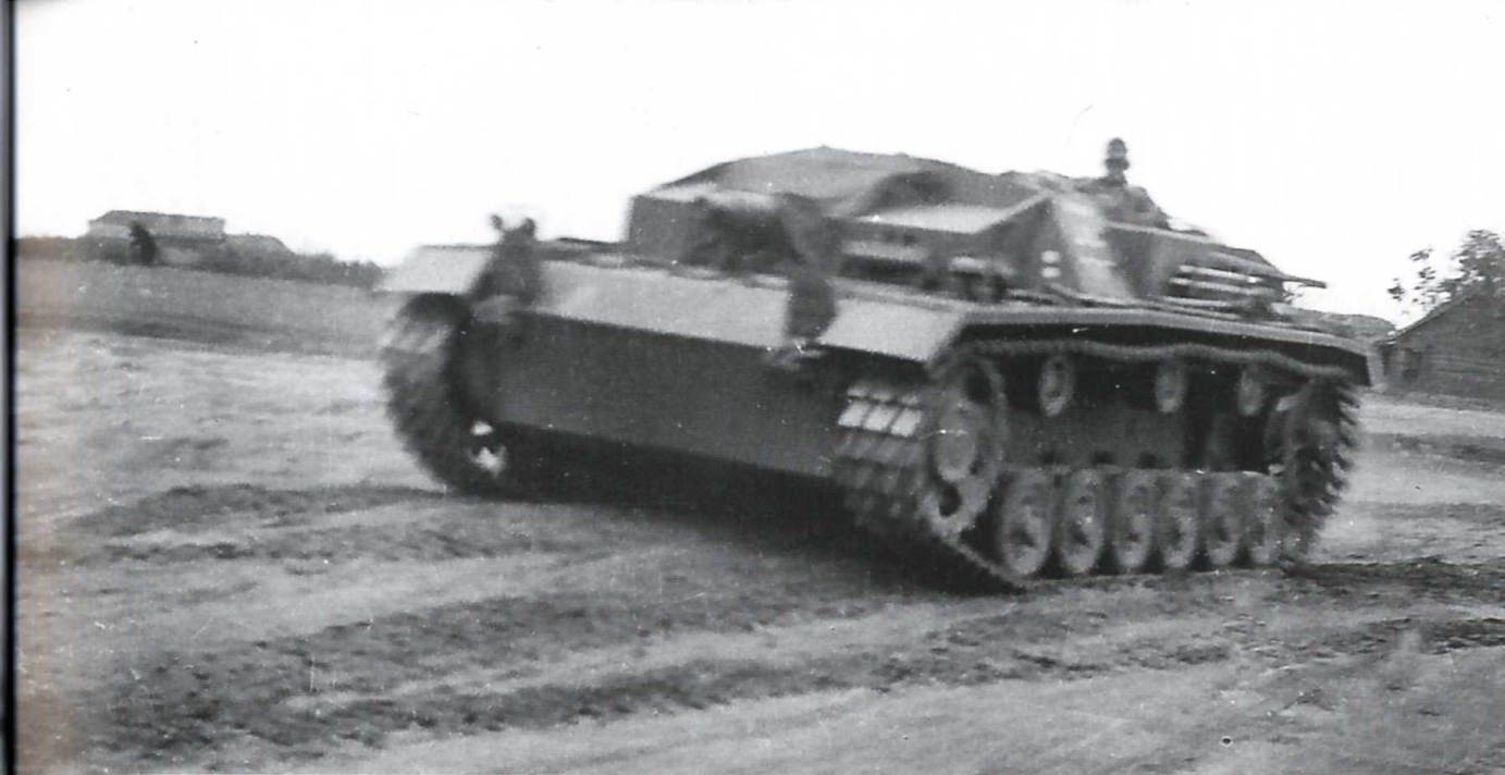
A StuG.III Ausf.B moves along a typical Russia road during the early victories on the Eastern Front. The crew have covered the part of the vehicle with a tarpaulin in order to keep dust out of the gun mantlet.
