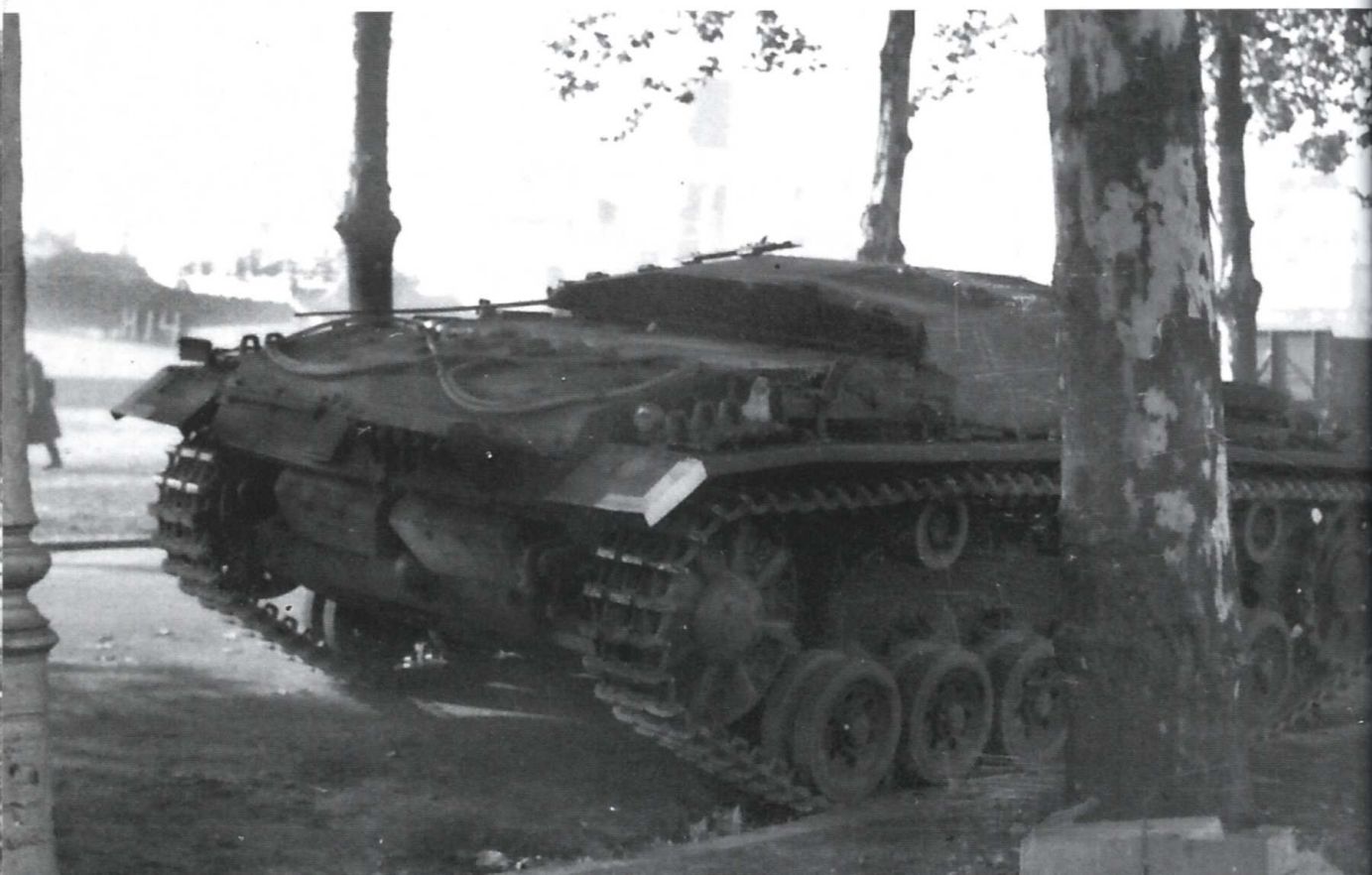
A StuG.III Ausf.B parked at the side of a road beneath some trees during the early part of the invasion of Russia in the summer of 1941. Note the white-painted edge of the rear mud-flap, which was used for low-light driving.
