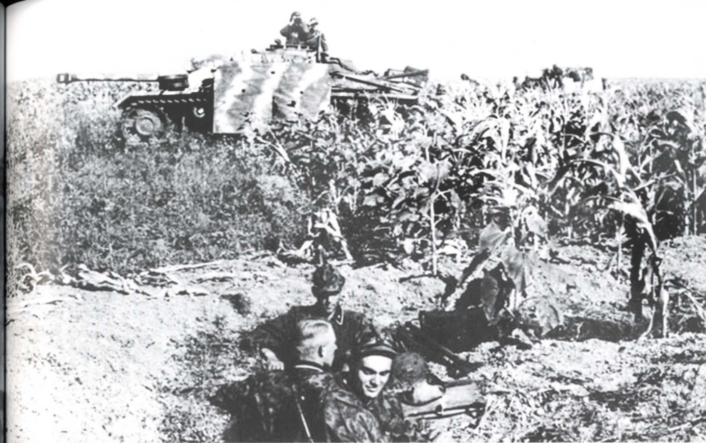
What appears to be a StuG.III.Ausf.G attached to a Waffen-SS unit. The assault gun has an interesting summer camouflage scheme of dark yellow base with bands of olive green. Note half of the armoured skirting which is missing following a contact with an enemy anti-tank shell.
