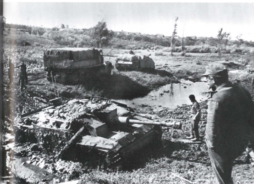
An Ausf.G moving along a road to the battle front in the autumn of 1944. Tank track links can be seen bolted to the casemate front plates. The vehicle has early type side skirting armour attached.
