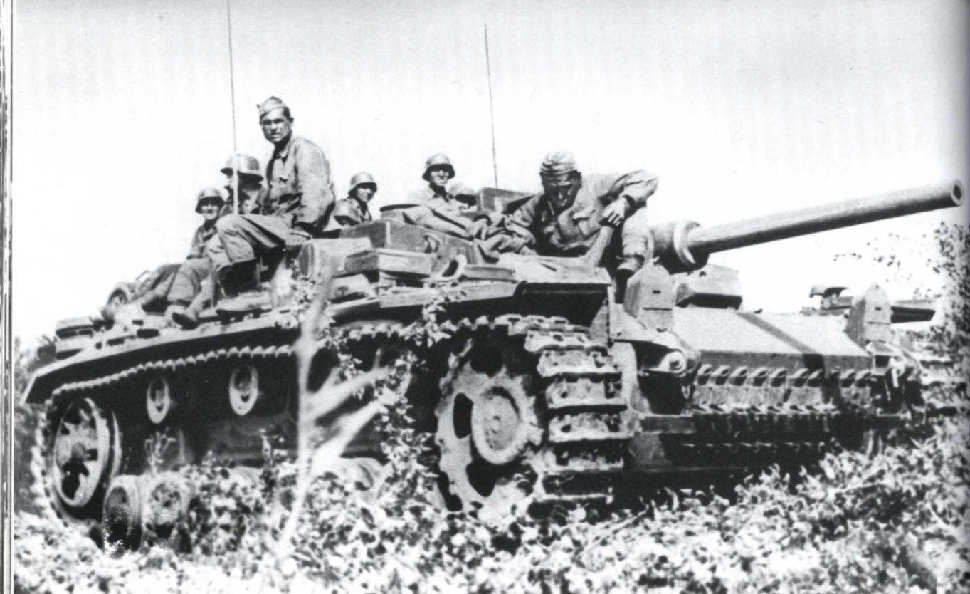
Infantry have hitched a lift onboard a StuG.III.Ausf.F. The vehicle displays two antennae, which indicates that it is a command vehicle. The assault gun is identified as a Ausf.F due to the long StuK40 L/48, but without the muzzle brake.
