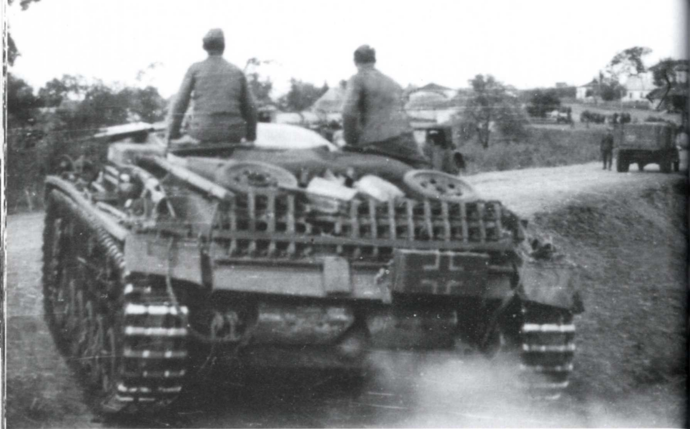
A rear shot of a StuG.III.Ausf.C/D as it climbs a small gradient in the road to join the vehicle column. As with many armoured vehicles in the late summer of 1941, many crews used spare track lengths and spare road wheels to create additional armoured protection.
