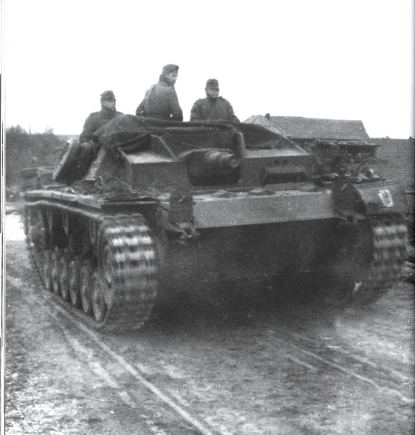
A StuG.III advances towards the battlefield. As with many of these vehicles because of its unique design there were many leaks and the crew often had to cover the fighting compartment with a specially fitted tarpaulin. Note the vehicle's unit marking on the left mud-flap indicating it belongs to the Sturmartillerie-Abteilung 189 .
