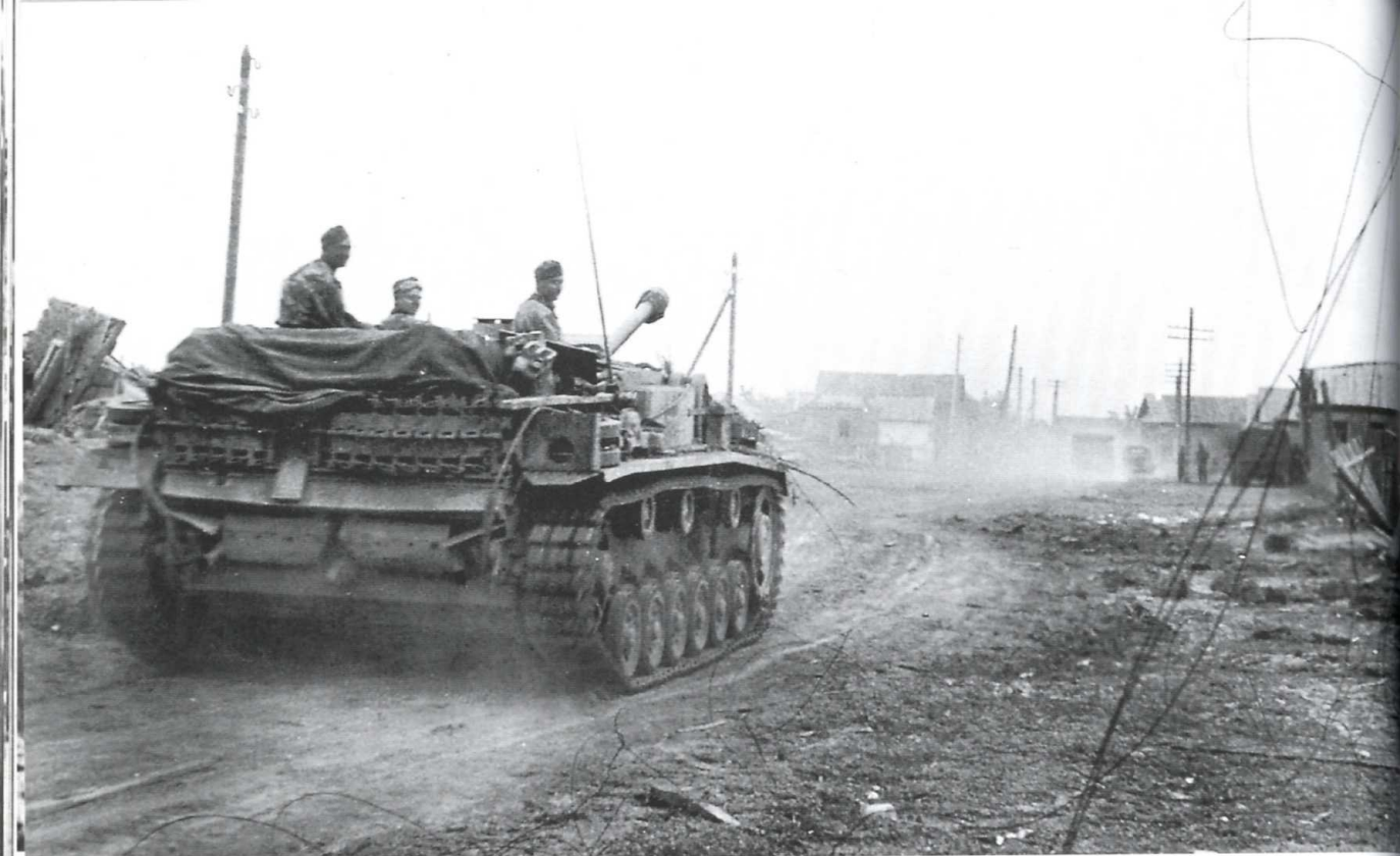
A StuG.III Ausf.F moves along a road most probably on the outskirts of Stalingrad in the late summer of 1942. The vehicle is fitted with the new StuK40 long-gun barrel, and the double-baffle muzzle brake. Note the track links bolted to the rear of the superstructure plate.
