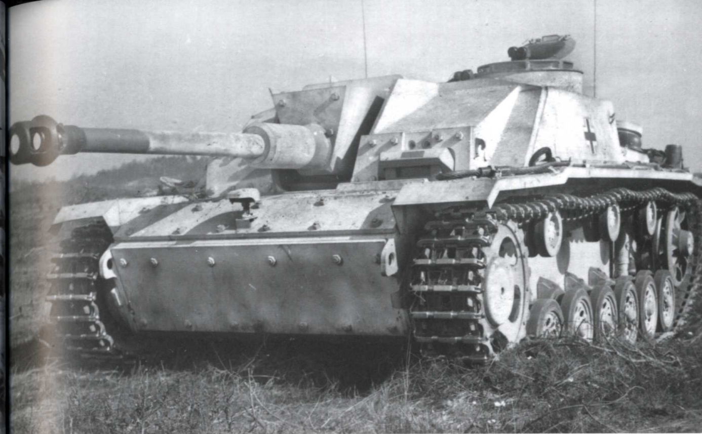
A new whitewashed StuG.III Ausf.G variant in a field. This was the final variant to be manufactured, and it came off the production line in 1943, and was rushed straight into service. The Ausf.G was armed with an MG34 for local defence and featured periscope to give the commander some protection as he surveyed the local terrain.
