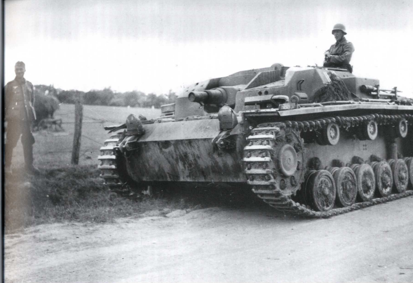
Two photographs taken in sequence showing a StuG.III has halted beside a road. This Ausf.B variant displays quite nicely its wider 40cm tracks, and by the appearance of mud and grass has undergone some cross-country driving. Note the Notek driving head-lamps mounted on the front of the vehicle. These lights could also be blacked-out.
