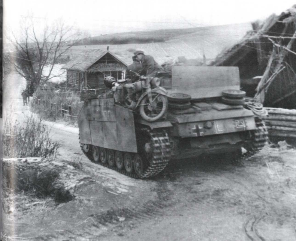
An Ausf.G moves along a road carrying a dispatch rider's motorcycle on the near track-guard. Note the markings on the superstructure rear plate, which is a sign for a tracked, self-propelled Panzerjäger unit.
