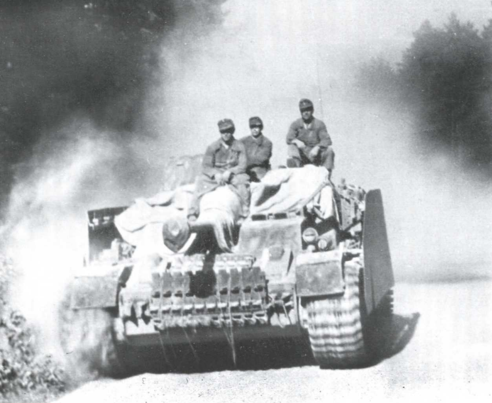
Crewman can be seen on their StuG.IV moving along a dusty road. Track links can be seen attached to the vehicle for additional armoured protection. Note the protective covering placed on the end of the 7.5cm guns muzzle break to prevent dust particles and other foreign matter contaminating the gun tube.
