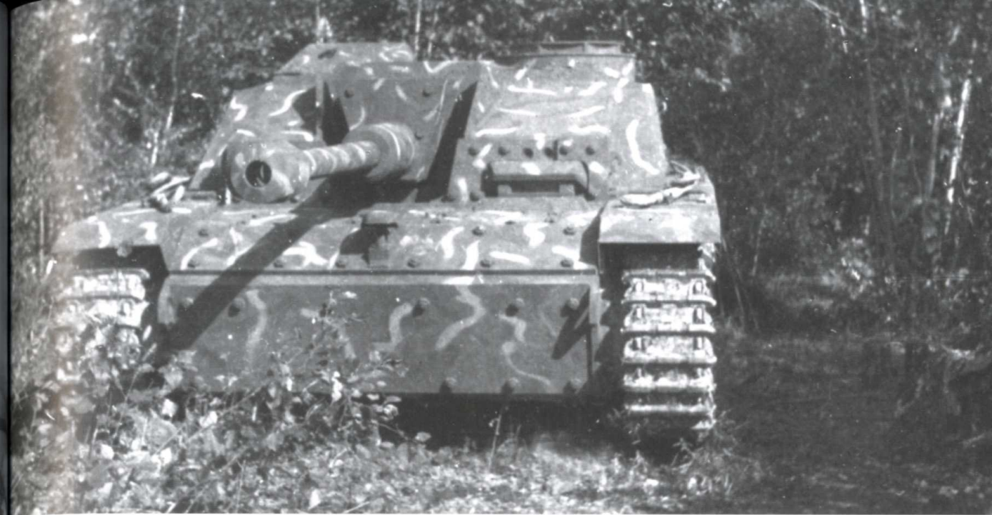
A StuG.III.Ausf.G in undergrowth. This vehicle displays a factory camouflage scheme of red brown or olive green with small stripes of dark yellow. The vehicle has been fitted with a folding shield for the loaders MG34.
