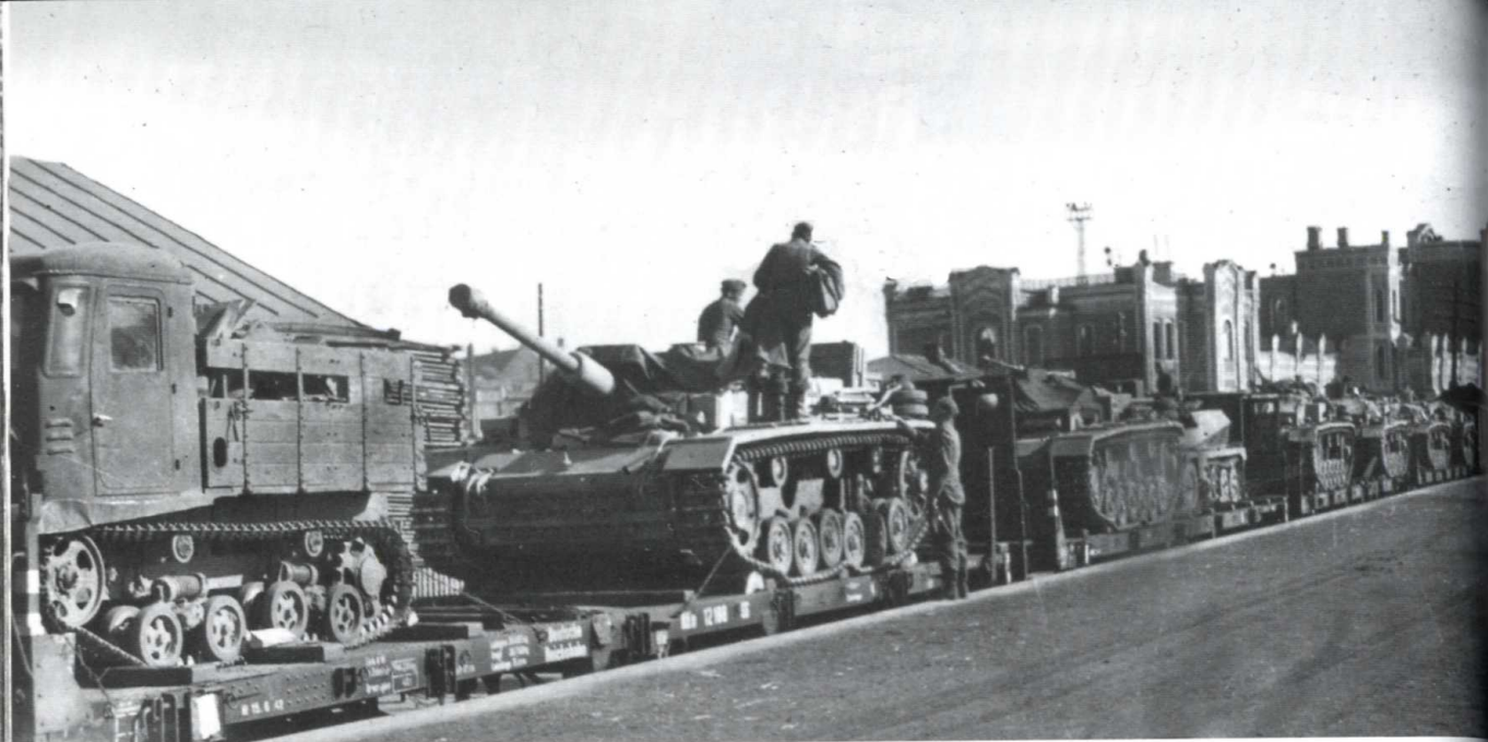
Two photographs showing a battery of StuGs on special flat-bed railway cars destined for the front. In typical German fashion these vehicles have been chocked and prepared for transportation. All retaining chains and cables are secured and in place.
